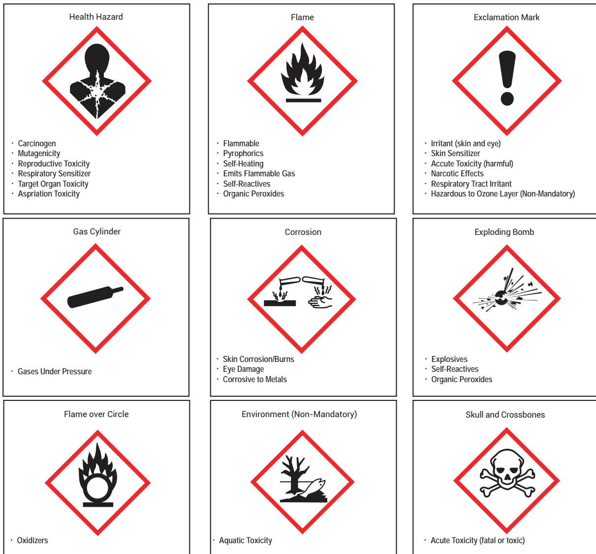
Figure 2: Pictograms (OSHA, Hazard Communication Standard Pictogram, 2020)
