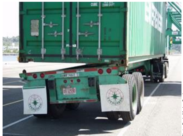
Semi-tractor with partially disengaged locking mechanism.
