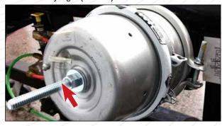
3. Loosen the clamp nut until the clamp band can be rotated.
