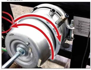
5. Tighten the clamp nut slowly, ensuring all housings and clamp band are generally centered. Tighten clamp nut to final torque of 25-31 ft-lbs. Check to see clamp is well-seated.
