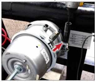
6. Remove caging tool and install in caging tool holder. Also, make sure the dust plug or Visi-Chek visual brake stroke indicator is installed on access hole of housing.
