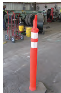
Figure 1: A typical work zone protection barrier; these barriers provide a visual sign that other vehicles should avoid the area.
