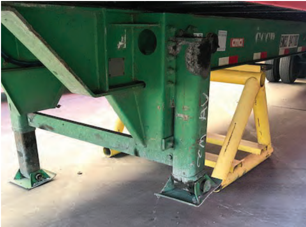
Figure 2: A chassis secured to level 4, supported on a stand specifically designed to support a chassis.
