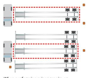
When performing minor repairs or inspecting a chassis, place work zone protection barriers as shown.
